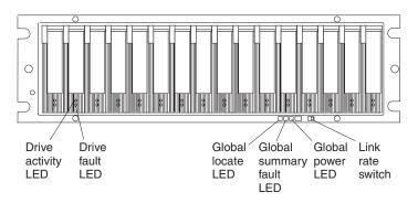
Figure 67. Front LEDs and controls
